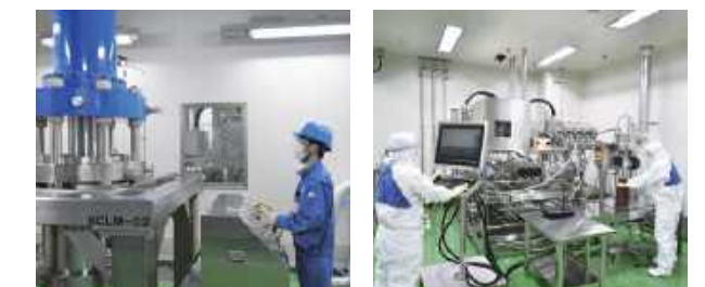
Chromatography system for the nucleic acid API purification plant
