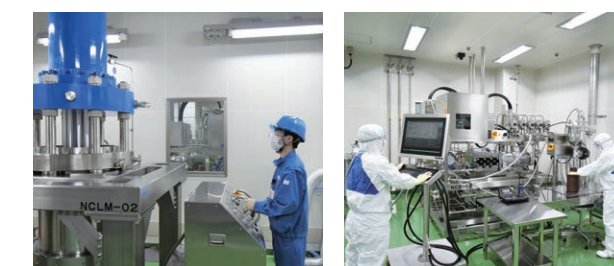
Chromatography system for the nucleic acid API purification plant
